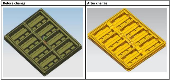
To remove the relay easily from the plastic tray, the HF115F-Q vertical plastic tray structure is fine-tuned. The external dimensions remain unchanged and the number of packages remains unchanged.
