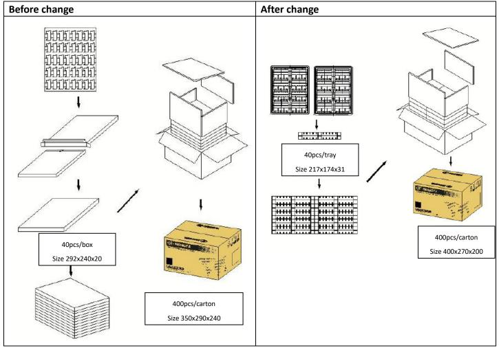
For the customer's convenience to take out the relay from the plastic tray, HF115F-Q horizontal type consists of a plastic tray + plastic bag The packaging of the carton is changed to the packaging of the upper and lower plastic trays to the cover (same as HF115F-Q vertical). Number of packages.
